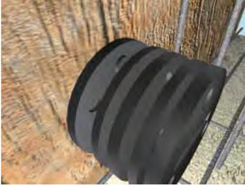
Cell-Cast® Interlocking Hole Forming Disks are designed to produce large diameter holes in poured concrete structures. Molded from non-conductive plastic, Cell-Cast® disks are lightweight and may be installed by one construction worker. They are available in a wide range of diameters using 3" and 4" thick modular disks.
