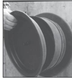
4. Place second end cap on sleeve. Check to determine that the cap is properly inserted.
