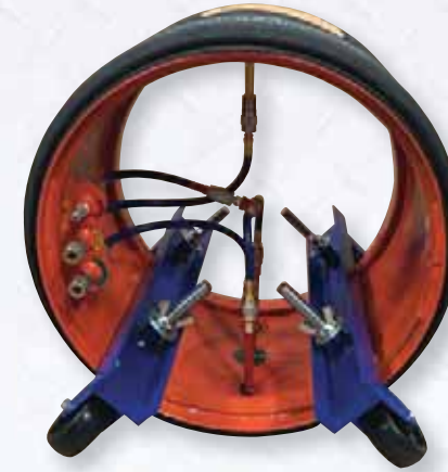
Custom 24" Joint Tester / Grouting unit. Designed built and shipped in 4 days.
